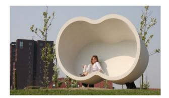
Binocular's design is a playful reference to field glasses. The benches provide both shelter and views that are sized to fit individuals and pairs. Metal structures raise the benches slightly, making them appear to levitate in the landscape. Binocular is made of reinforced cast stone.
